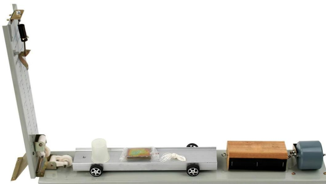
This [Friction Apparatus, Advanced](#) type is used to demonstrate static friction, sliding friction and rolling friction. Students can investigate friction qualitatively and quantitatively. This [Friction Apparatus, Advanced](#) type includes:
