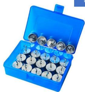
Hooked Weight Set for General Science and Physics in Mechanical Balances, 20g x 20pcs, Chrome Plated Iron, with Storage Case
